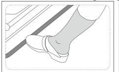
Control takes place by means of moving the walking-free foot control vertically (up or down) with a foot. The walking-free foot control is located around the base of the table.
