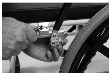
Attach the brake to the frame
