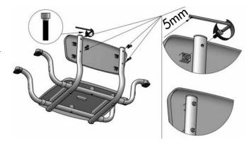
**Step 6.** Check if all elements were assembled correctly and the bench width was adjusted correspondingly to the bath width.
