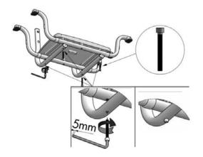
Note! Ensure the elements of backrest frame are mounted at the back of the seat – the rear part of the seat is narrower than the front part.
