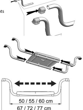
**Step 2.** Fix side frame elements into the mounting openings on both sides of the seat.
