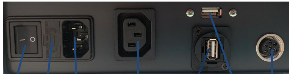
Switch ON/OFF general Tray fuse holder Three-pole socket for cable diet Socket for trolley power cable (not in use) USB connector, cart data connection (not in use) Connector for connection of USB pendrive Pedal connector (not in use)
