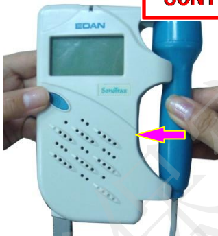
Figure 3-5 Placing the probe
