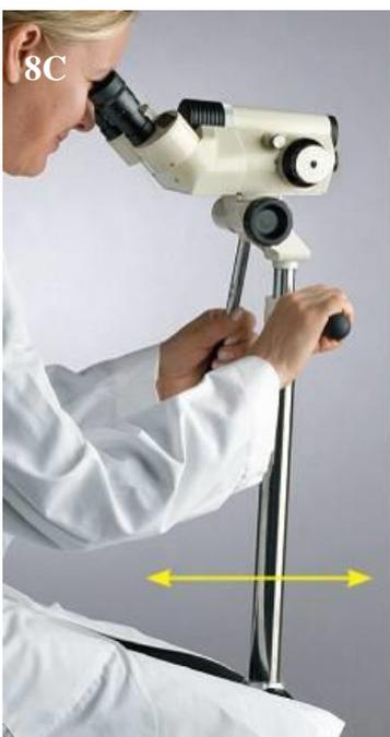
C. With your right hand on the Fine Height Adjustment Handle, slowly push or pull the Colposcope, until the field comes into view.
