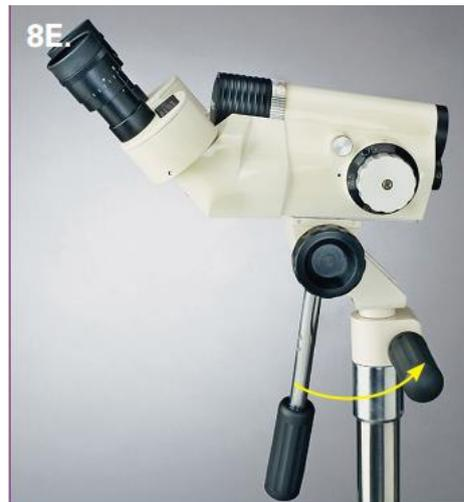
Push the Fine Height Adjustment Handle forward and to the left (counterclockwise).
